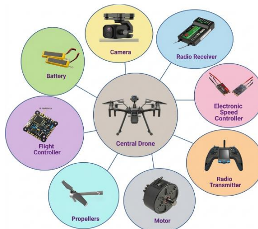
Fig. 2. Essential elements of drones utilized in agricultural operations
